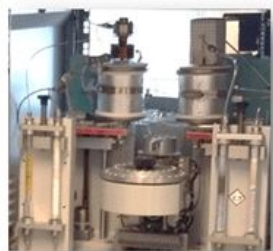
SOC thermal fractionation using Rock-Eval®
